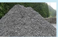
We're currently examining the collection, treatment, and recycling the fly ash generated from fuel used in thermoelectric power plants as materials for road paving.
