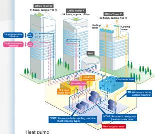
A pump that uses a small amount of electricity to pump renewable heat included in natural air, water, etc. instead of using combustion. Makes it possible to use heat equivalent to three to six times the electrical energy input
