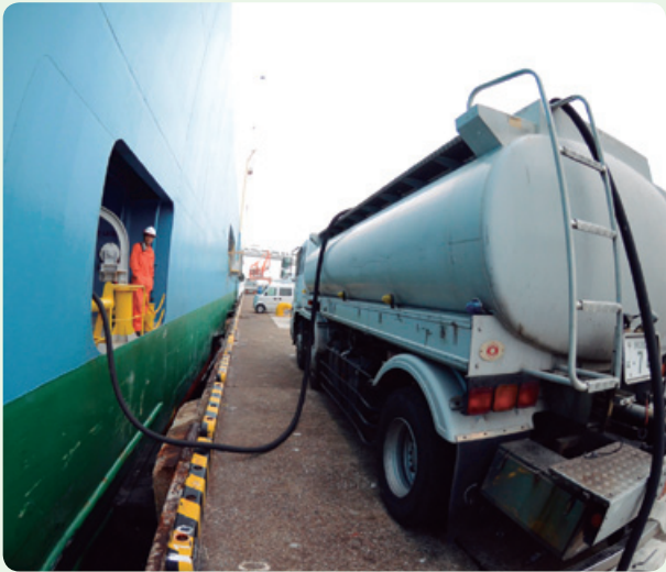
Sludge (unburned waste oil) from fuel tanks of ships can be recovered and processed, and subsequently put to use as recycled oil. The photo shows the recovery process of transferring sludge from a ship into a tanker truck.
