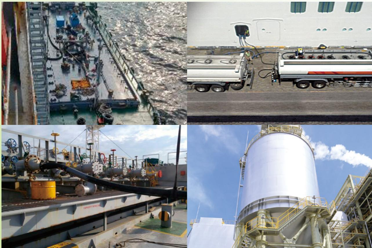
Upper/lower left: Slop is collected by connecting outbound oil tankers to collection craft by hoses. Upper right: Sludge (unburned marine fuel) collected from shipboard sludge tanks can be treated and used as a recycled oil source. This photo shows sludge being loaded from a ship to tanker trucks. Bottom right: Sendai Power Station Co., Ltd., operates fly ash storage facilities.
