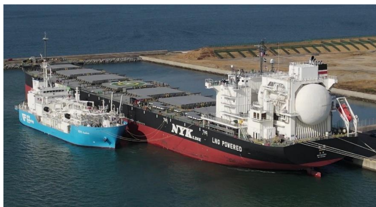
LNG bunkering operation by KEYS Azalea (December 2024)
